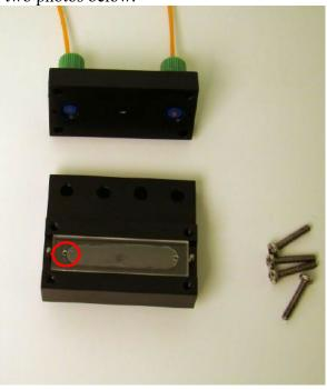
Warning: Holes must face upwards.
