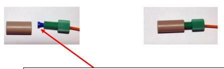
Blue Ferrule must be pre tightened onto the tubing before using in the USP flowcell. This is easily done by first mounting the ferrule and nut into any available ½-28 flat bottom port such as the included union (as pictured). Tighten nut into union and then remove. The blue ferrule should now be tight on the tubing. The tubing should be flush with the end of the blue ferrule.
