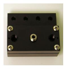
3) Pretighten/collapse the blue ferrule onto the tubing. This step is performed because it takes some force to tighten the blue ferrules, a process that could crack the slide (step 5). So the blue ferrule must be pre-tightened using a different \(^1/4\)-28 port.
