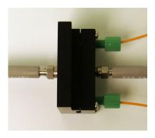
The SMA-USP Flowcell - The new SMA Ultra-Short Path Flowcell allows absorbance measurements through an optical path length as short as 100 microns. Available optical paths are 100, 200, 500, 1000 and 2000 microns. Others may be available upon custom requests.
